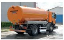
panel, allowing turning on and off individual flushers and switching on warning lights. Flushing takes place by means of aluminum flushers (featuring individual turning on and off from the cab). Sprinkling takes place by means of a spraying beam.
