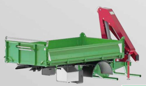
3WBH tipper + crane - for the construction industry
