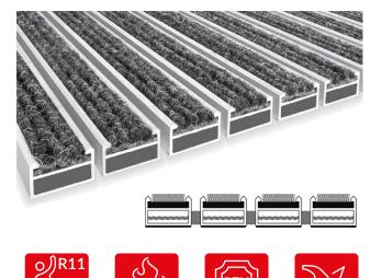
Entrance mat with drying cleaning inserts in an aluminum profile. Drying inserts are abrasion and compression resistant, and absorb moisture well. Units/profiles are held together by stainless steel wire. Designed for entrances with normal (12 mm high) to heavy (17 or 22 mm high) pedestrian traffic, forklifts and shopping trolleys (22 or 27 mm high mats). For indoor use only.
