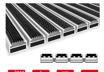
Entrance mat with rubber cleaning inserts in aluminum profiles. Units/profiles are held together by stainless steel wire. Designed for entrances with normal (12 mm high) to heavy (17 or 22 mm high) pedestrian traffic, forklifts and shopping trolleys (22 or 27 mm high mats). Rubber cleaning inserts have a high mechanical strength and are resistant to moisture, corrosion & temperature changes.
