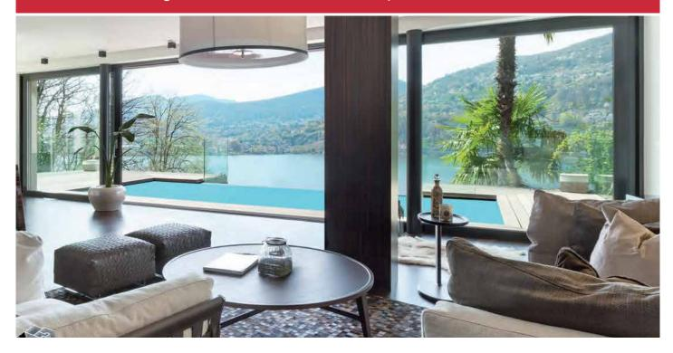
The **ULTRAGLIDE** system meets the current standards in the field of safety, thermal insulation, and aesthetics. Great parameters of the **ULTRAGLIDE** system allow to design large constructions even up to 16 meters width with maximum achievable dimensions of sash height 3300 mm and sash width - 3500 mm (max sash weight 250 kg for the sliding option, and 400 kg for the lift-and-slide option). This system allows your imagination to come true about the largest sliding doors.
