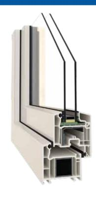
System Perfectline 70 characterized by 5 chambers in the frame and 5 chambers in the sash with an installation profile depth of 70 mm is created to provide heat insulation at a high level. A system of two external gaskets ensures good tightness, acoustic insulation. Gasket surfaces with a 15 degree gradient enable very good drainage of water and dirt.
