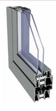
The **Imperial I+** profile system features good insulation parameters (Uf from 1.28 W/m²K). High thermal insulation parameters are obtained by using special thermal inserts between the thermal separators and around the glass pane. This system allows for the use of all common types of single-, double-chamber, acoustic or anti-burglary glass despite the profile installation depth of only 65 mm.
