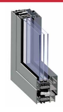
**Genesis** aluminium system designed for windows and doors with increased thermal insulation (U<sub>f</sub> from 0.84 Wm<sup>2</sup>K). This three chambers profile uses modern thermal break solution, which are currently a novelty on the market. Apart from the classic central window gasket, an additional thermal seal was designed, as a result of which a very high tightness was obtained (air infiltration, watertightness) along with an innovative appearance and aesthetics.
