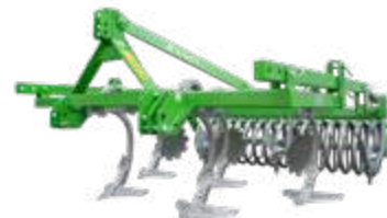
Overload protection by spring tooth
